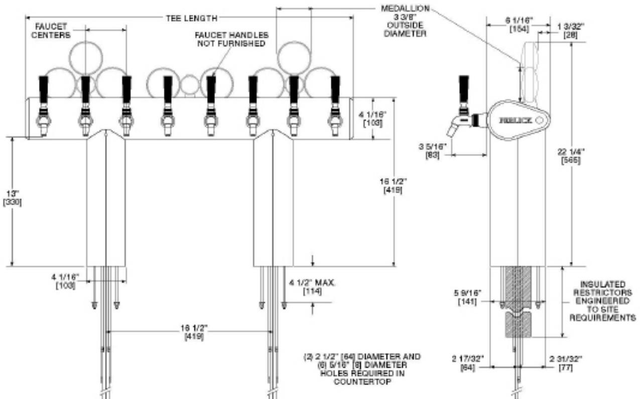
MODEL NUMBERS - 66500-8B, 66500-10B, 66500-12B, 66500-8BPC, 66500-10BPC, 66500-12BPC, 66500-8BTF, 66500-10BTF, 66500-12BTF, 66500P-8BIM, 66500P-10BIM, 66500P-12BIM, 66500P-8BPCIM, 66500P-10BPCIM, 66500P-12BPCIM, 66500P-8BTFIM, 66500P-10BTFIM, 66500P-12BTFIM
