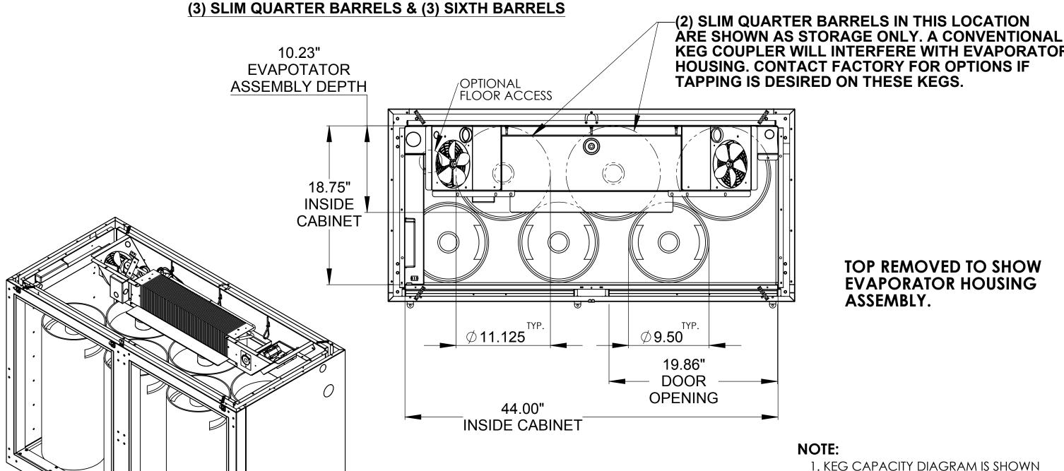
**KEG COUPLER WILL INTERFERE WITH EVAPORATOR** HOUSING. CONTACT FACTORY FOR OPTIONS IF TAPPING IS DESIRED ON THESE KEGS.
