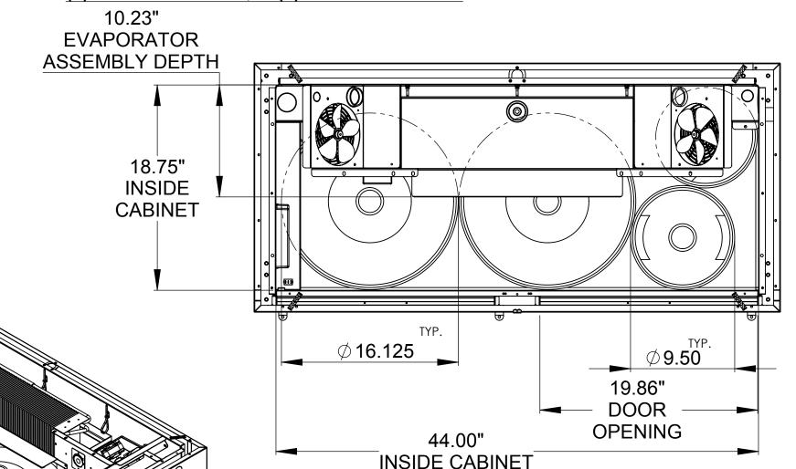
TOP REMOVED TO SHOW EVAPORATOR HOUSING ASSEMBLY.
