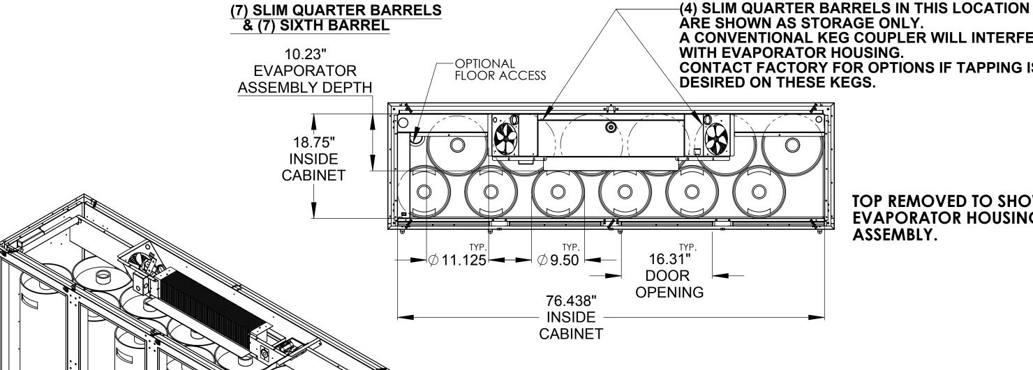
ARE SHOWN AS STORAGE ONLY. A CONVENTIONAL KEG COUPLER WILL INTERFERE WITH EVAPORATOR HOUSING. **CONTACT FACTORY FOR OPTIONS IF TAPPING IS DESIRED ON THESE KEGS.**
