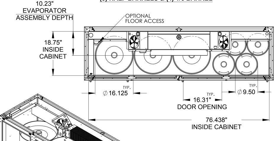
TOP REMOVED TO SHOW **EVAPORATOR HOUSING** ASSEMBLY.
