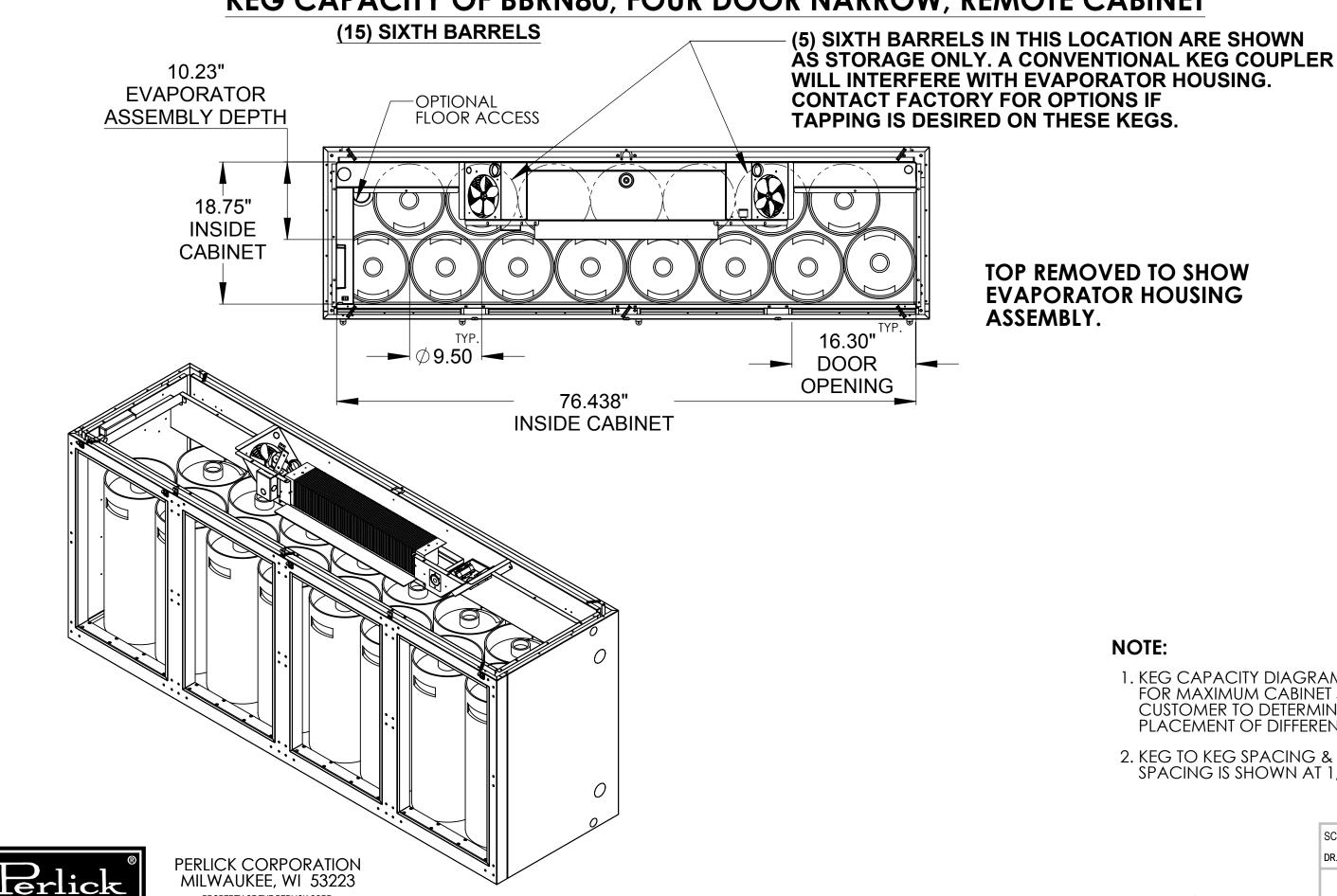
TOP REMOVED TO SHOW **EVAPORATOR HOUSING** ASSEMBLY.
