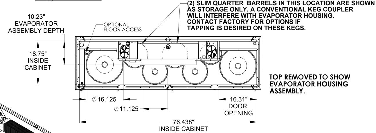
TOP REMOVED TO SHOW **EVAPORATOR HOUSING** ASSEMBLY.
