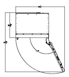
Max clearance required for opened door is 49-3/4'' when opened to  $90^{\circ*}$  (dimensions shown are without door overlay installed.)
