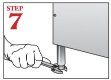
Level the glasswasher by adjusting the leveling legs. Both the front and back of the glasswasher must be level to operate correctly.
