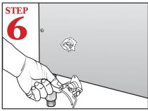
After filling the glasswasher for the first time, (CAUTION: Turn power supply off) connect the wire to the booster high-limit switch located behind the front panel, as shown.
