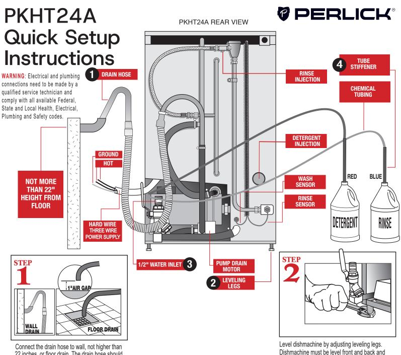
22 inches, or floor drain. The drain hose should have a 1 inch air gap between drain hose and drain.
