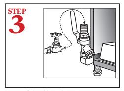
Connect dishmachine to hot water source, recommended minimum temperature 140°F. Unit will remain in wash cycle until booster heater temperature reaches 180°F, then it will advance into rinse cycle.
