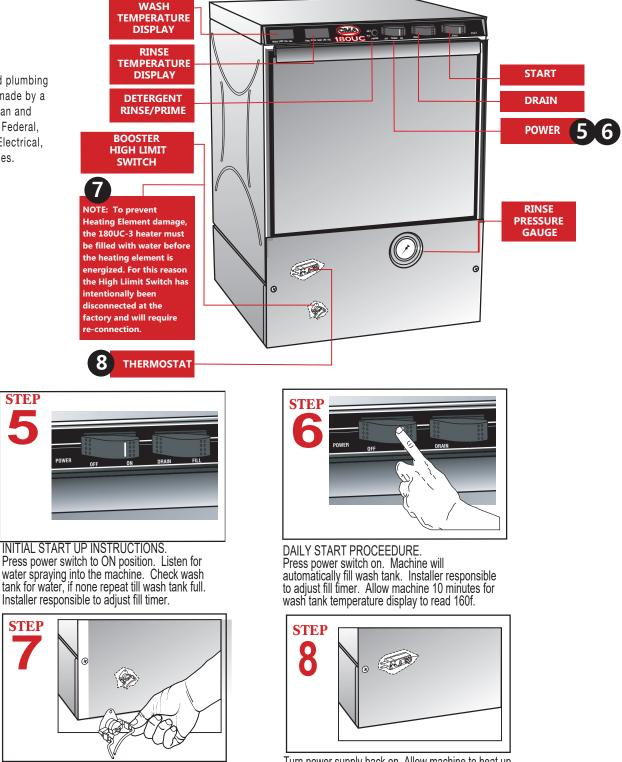
After filling dishwasher for the first time, (CAUTION: turn power supply off) reconnect the factory unplugged wire to booster high-limit switch located behind front panel.
