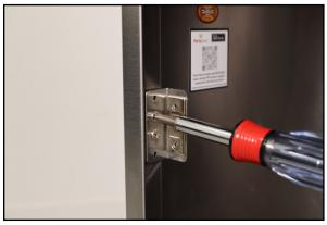
7) Position the hinges in the pre-punched holes on the opposite side of the door frame.
